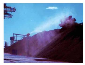
controlled in a centralized control room, and can calibrate their direction for optimal throw based on the current wind conditions. HKD Blue
