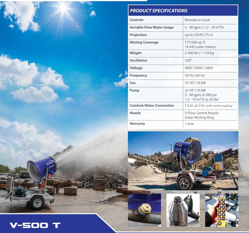
Just like all HKD Blue V-500 models, the V-500 T has a powerful 25HP fan, 25 HP booster pump, our Variable Flow Central Nozzle, outer misting ring, onboard pressure washer, and full remote control functionality. This unit comes on a 7'x6' DOT certified galvanized trailer which is ideal for maneuverability from one job site to another.
